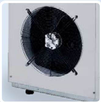
Corrosion proof peraluman body, axial fans with outside rotor and low rotations number, microprocessor-based electronic control et antivibration rubber mounts.
